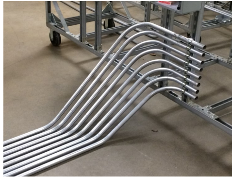
Third year apprentices working on their conduit bending skills at the Training Center.
